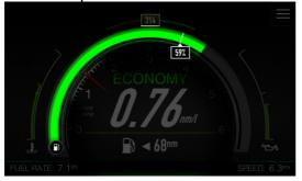
When a fluid level sensor is connected to network, green arc will display averaged measured quantity and white pointer will show calculated fuel.
