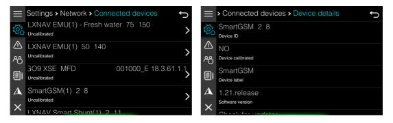
Select a device to get more details about it. At the bottom of the device details, there is an option to reset configuration for this device. This will delete all configurations previously done for this device and device will behave as being seen for the first time.
