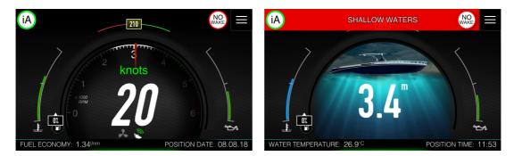
When IAssist screen is displayed, green icon with iA label will be drawn in top left corner of the screen. Press it to dismiss IAssist screen.
