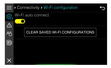
Press CLEAR button to delete all stored Wi-Fi access point configurations.
