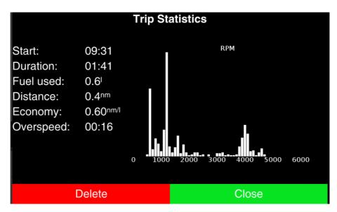
Start of current trip and its duration. Duration is taking into account only time, when engine was running. Fuel used during trip. Distance covered. Fuel Economy, which is calculated based on distance covered and fuel used during duration of this distance being done. Overspeed time is time, when vessel was travelling about set high speed and above no wake
