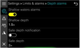
On your device you can set two different depths. First one is call safe depth and the other one is called shallow waters. This allows you to setup two stage depth warnings.
